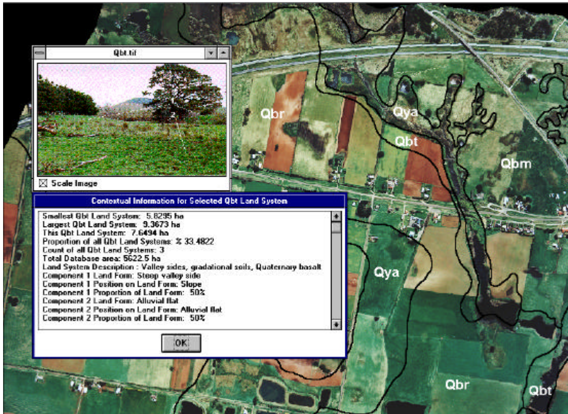
Figure 3: A "Smart Map". Note the photogrammetrically correct (colour) aerial photography used as a backdrop to the Land System polygon boundaries. These are the photos from which the Land System theme was derived. The insert is a three dimensional representation of a Land System block diagram with component tags placed in accordance with Jeffery's component description. Note in that the area depicted needs to be relatable to the area as a whole, it is important that both contextual statistical and descriptive information is available (see box).
