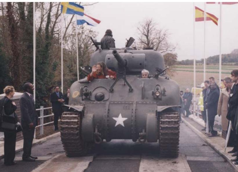
A truly extreme test: A Sherman tank is driven over Westmill Bridge, a state-of-the-art structure into which 40 fibre optic sensors have been incorporated. The sensors will continually monitor the strain the bridge is under during traffic flow and any extreme events.
