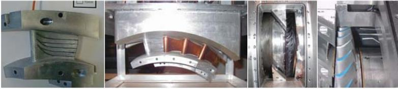
Left: Optical fibres embedded in a jet turbine assembly can be routed to the exact point at which measurements need to be made. Data gathered from these sensors during tests show engine emissions and efficiency.
